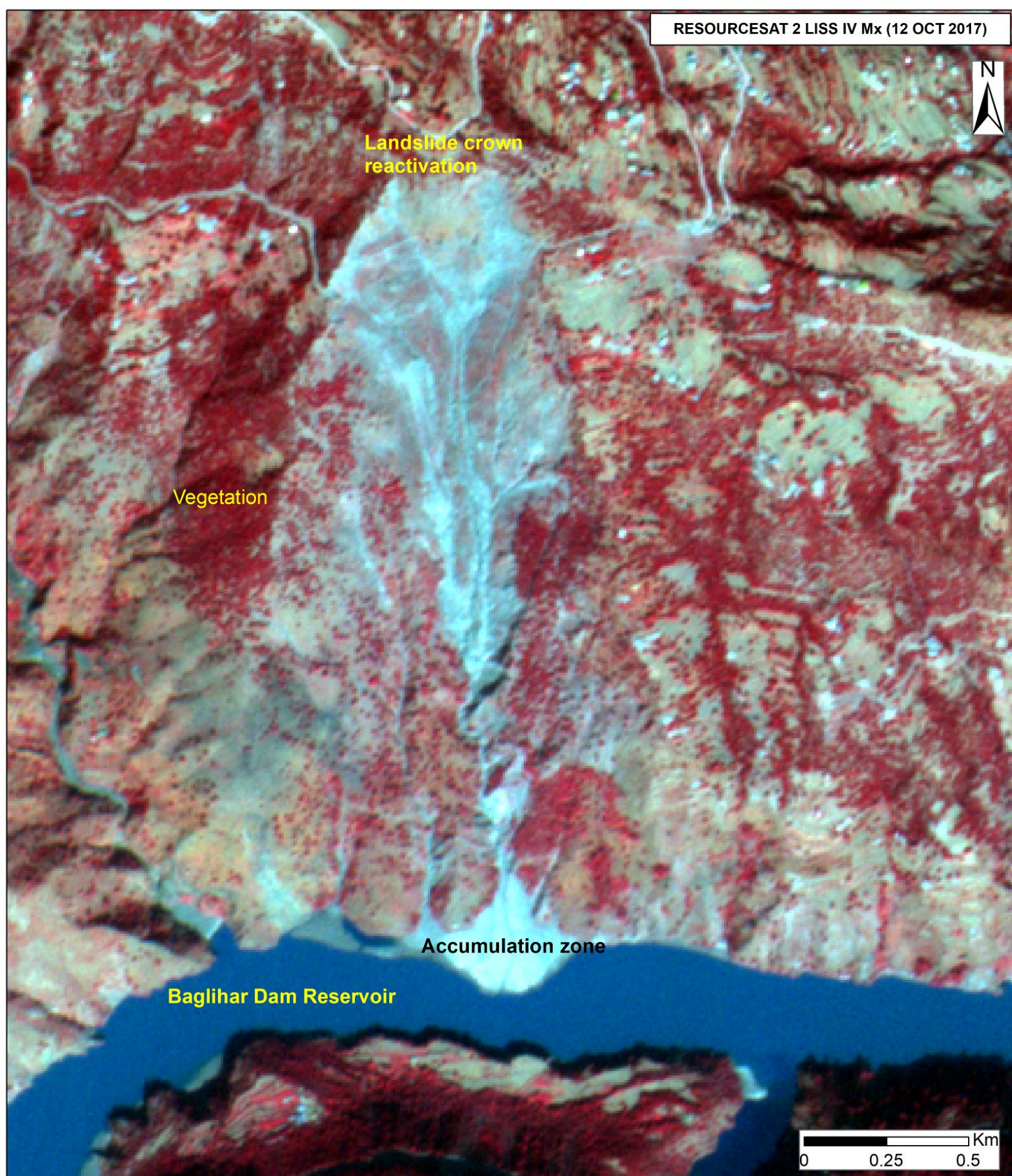
Figure 12. Paryote landslides near Paryote village in Doda district, Jammu and Kashmir. The continuous reactivation of Paryote Landslide near Paryote village in Doda district of Jammu and Kashmir. Translational-type failure with rock fall has occurred near the crown of the landslide, followed by a partially channelized debris flow along the main body of the landslide.
